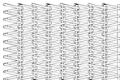
Fig. 1 — Balanced Weave wire mesh conveyor belt with specification B-30-16-10-12
