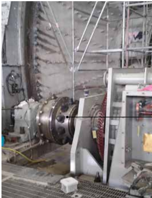
Pictured above: An Autogard 820 Series Torque Limiter installed in a ball and SAG mill mining application.
