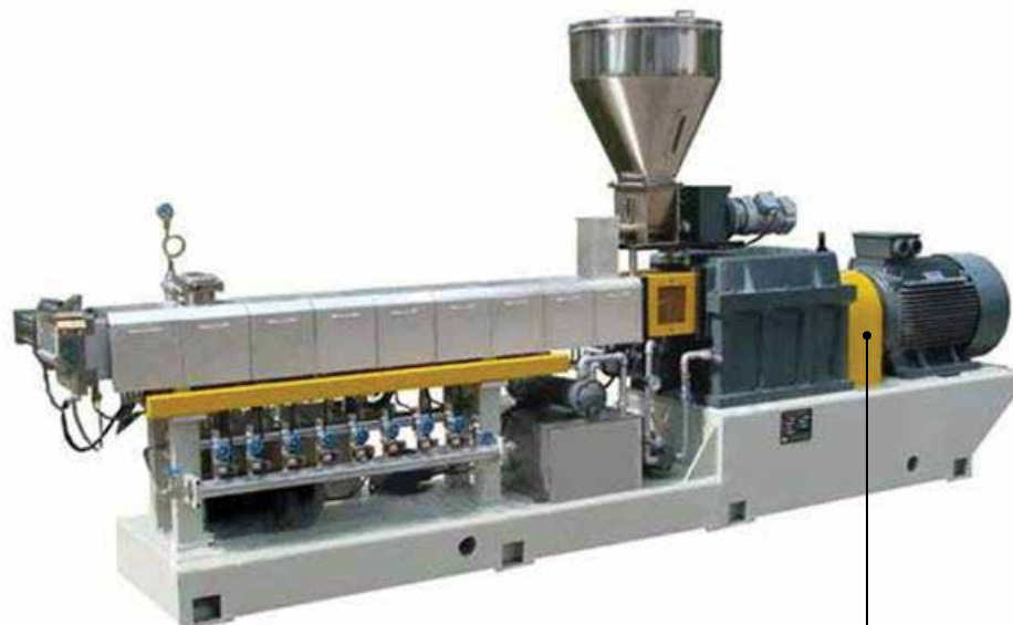
Torque limiter and coupling between motor and gearbox
