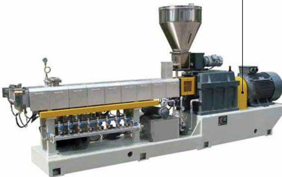
Torque limiter and coupling between motor and gearbox
