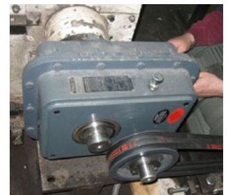
A Falk Quadrive with the proper service factor was installed, delivering 94% savings per year.
