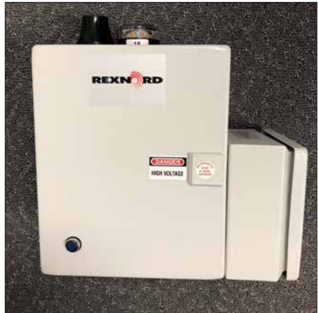
Figure 13 – Edge device assembly with optional cellular antenna and Andon light
