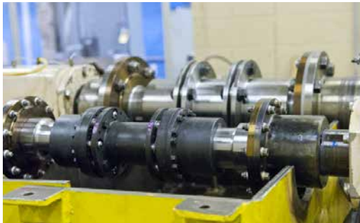
Four square coupling test
