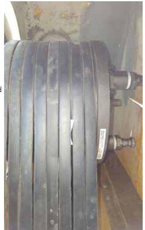
Cone crusher application showing v-belt pulley with Autogard connection.
