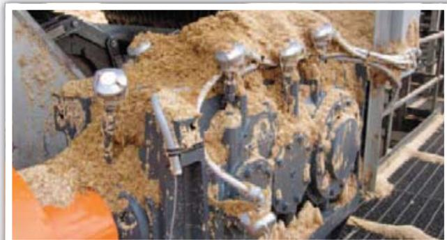
**After three months of 24/7 operation with heavy debris buildup, the new drive was running quietly, with excellent gearing contact and sump temperatures in the 140°F (60°C) range, despite high ambient temperature and humidity. The temperature of the drive did not change dramatically from a "clean" housing to the conditions shown above. On one typical day, with the outside temperature at 97°F (36°C), the sump was running at less than 150°F (65°C) degrees, despite a heavy buildup of debris.**
