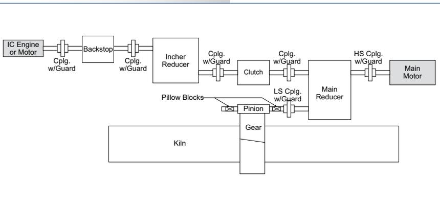
Figure 1 - Typical Kiln Inching System
