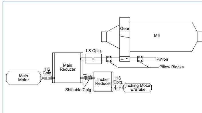
Figure 2 - Typical Mill Inching System
