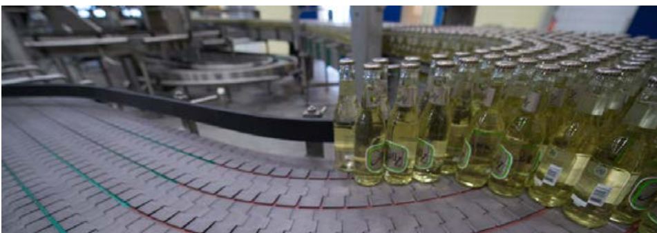
The Rexnord Combi-X Corner Track System is equipped with the proven Rexnord Combi Chain retention design.
