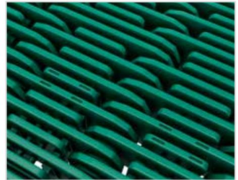
**New marking on the top surface of the belt to determine position of the Positrack® guiding lugs, without the need to open the chain.**
