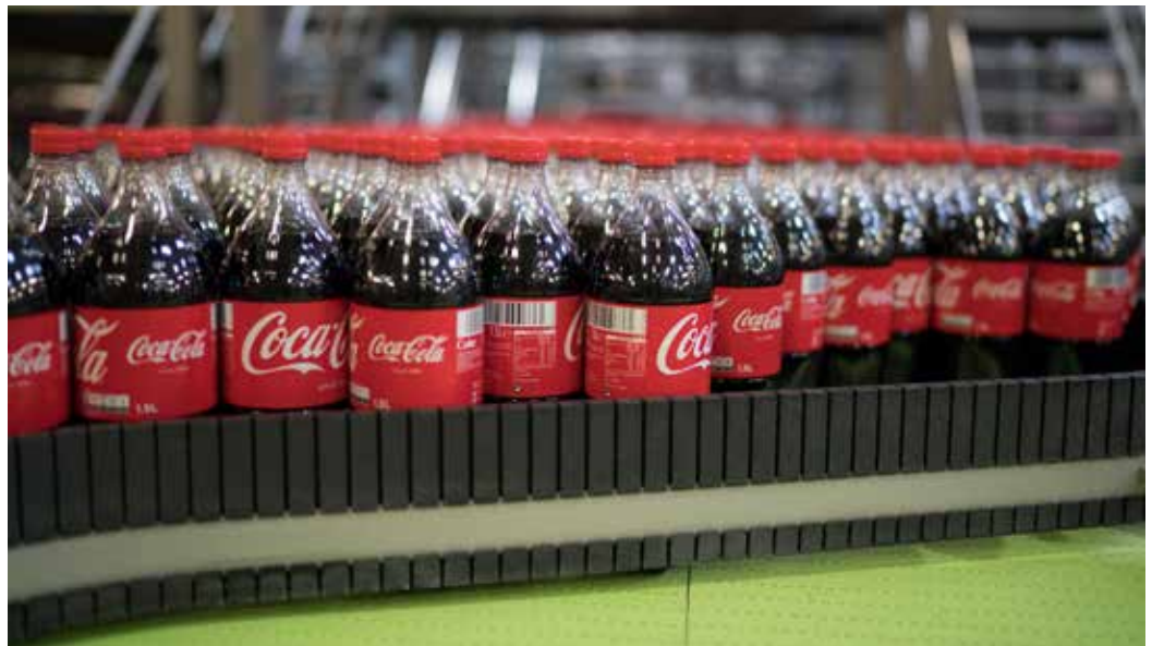
Conveyor equipped with Rexnord 1000 Series FlatTop in DRY-PT material
