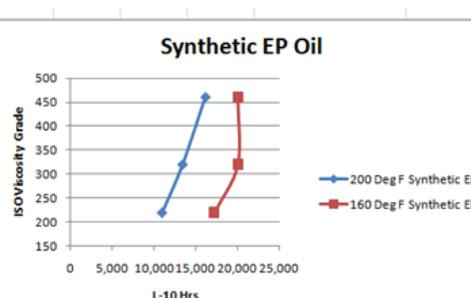
Note a maximum limit of 2.5 x Base L-10 hrs was applied to the lubrication factor.
