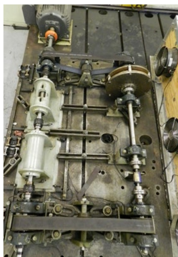
Figure 2 – Operating under misalignment test stand
