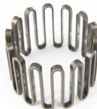
Dodge grid element after 70,000 cycles
