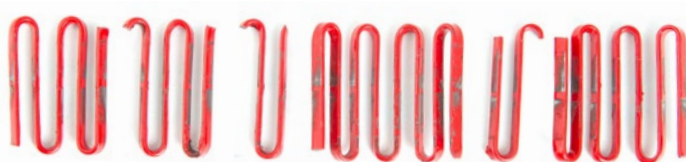
Dodge grid element after 70,000 cycles
