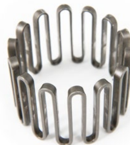
Dodge grid element after 70,000 cycles
