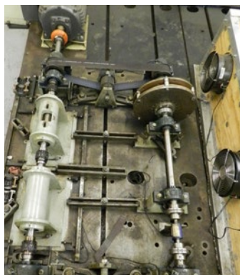
Operating under misalignment test stand
