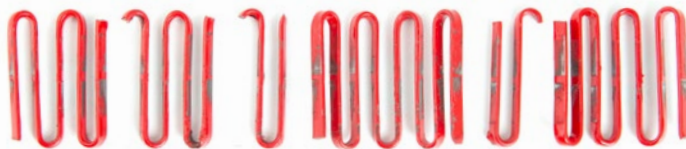
Dodge grid element after 70,000 cycles
