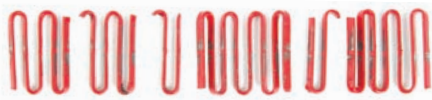
Dodge grid element after 70,000 cycles
