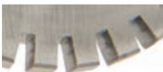
After 400,000 test cycles, Falk Steelflex hub shows no wear with smooth, machined surfaces.
