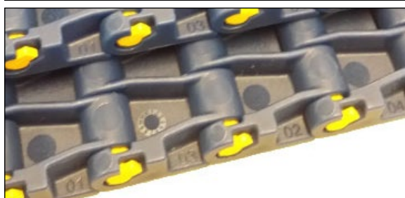
Upgraded Design with 1500 Plugs on Both Sides of the Belt
