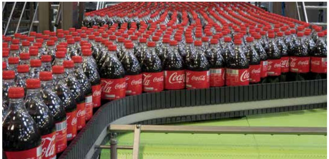
High-speed PET filling line, equipped with Rexnord MatTop chain in Dry-PT material
