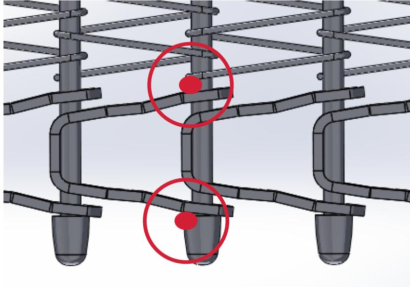
9. Continue to install successive belt sections in a similar manner until all the spiral conveyor has been fully loaded with new belt.
