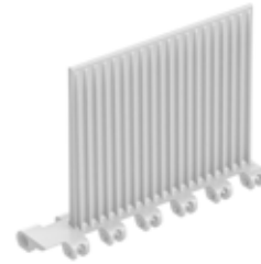
Rexnord 1010 Series KleanTop Belt Ribbed Flight 6-inch width, 4-inch height, 1-inch side indent
