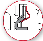
Rex Z Seal Non-Contact Seal
