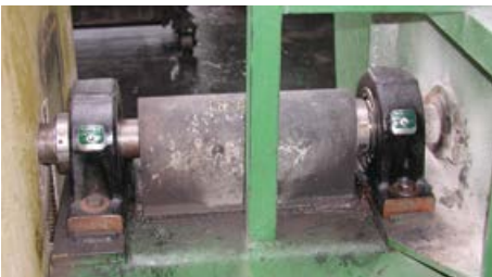
Link-Belt H Seal Clearance Seal
