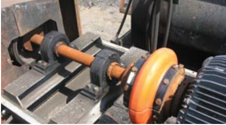
Rex Z Seal Non-Contact Seal
