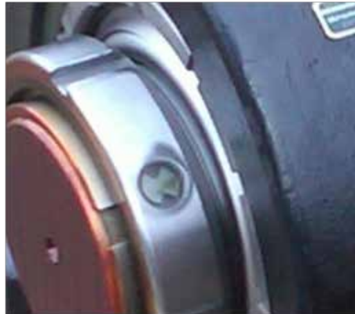
Spyglass Optical Strain Sensor (OSS) technology lets the mechanic know when correct tightness is reached.
