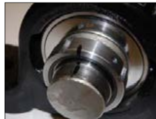
Figure 2 — Position of Locknut relative to shaft
