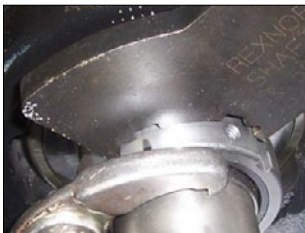
Figure 1 — Wrench positioning to prevent sleeve from slipping
