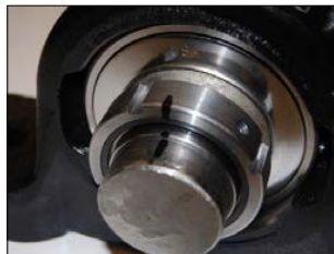
Figure 2 — Position of Locknut relative to shaft
