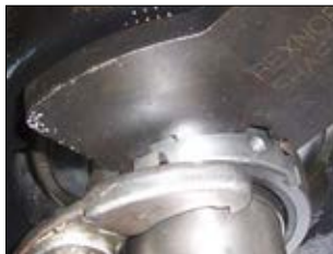
Figure 1 — Wrench positioning to prevent sleeve from slipping
