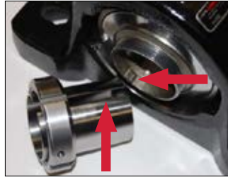
Figure 3 — If sleeve is removed from inner ring align spline with slot in sleeve to reinstall
