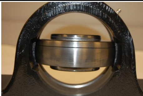
Figure 3) Loading bearing into loading slots
