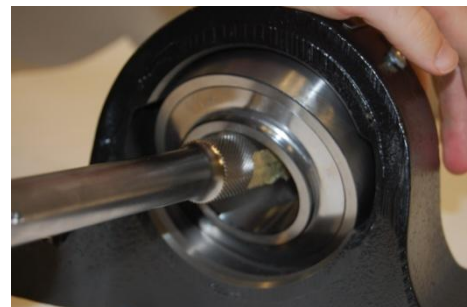
Figure 4) Torquing bearing 90° into housing
