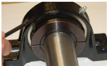
Figure 1) Set screw tightening on a Centrik-Lok bearing
