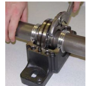
Figure 2 — Tighten Until Snug
