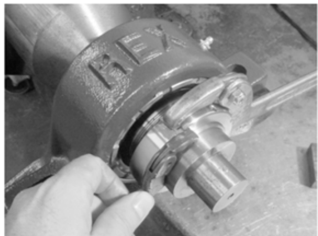
Figure 1 — Wrench positioning to prevent sleeve from slipping
