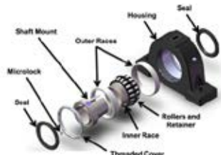
Figure 6 — Exploded view Rex Shurlok
