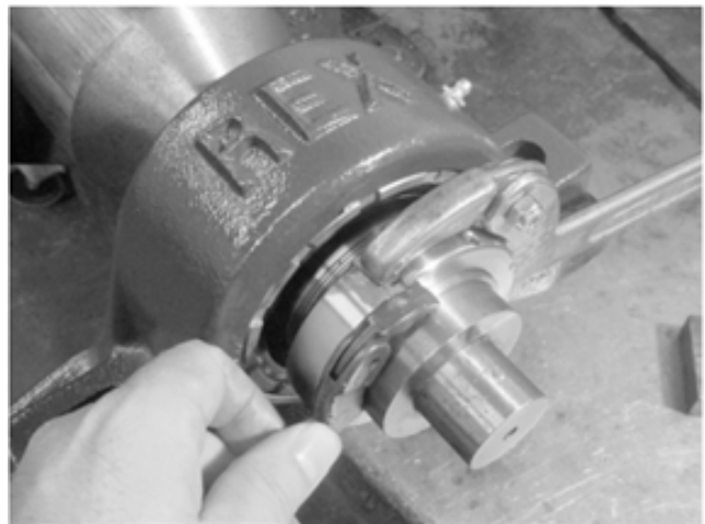
Figure 1 — Wrench positioning to prevent sleeve from slipping
