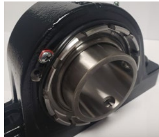
Figure 3 — Proper O-Ring Installation
