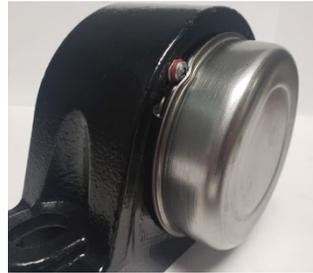
8. Press cap over threaded cover. Using a rubber mallet apply force to the cap to properly seat cap over the threaded cover. Some deformation of the cap around the microlock assembly is to be expected (Figure 4).
