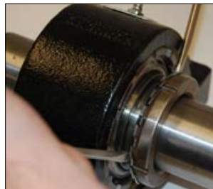
Figure 1 — Zero Shaft Fit Pry against housing to draw adapter sleeve through bearing. Sleeve should not be protruding out the backside of the inner ring.
