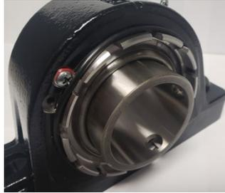
6. Turn housing over and provide support so inner race on threaded cover side sits above table. Place a soft piece of steel or block of wood that just fits over the face of the inner ring. Using a soft blow hammer, strike the block with several sharp blows, inner ring assembly should rotate and misalign freely.
