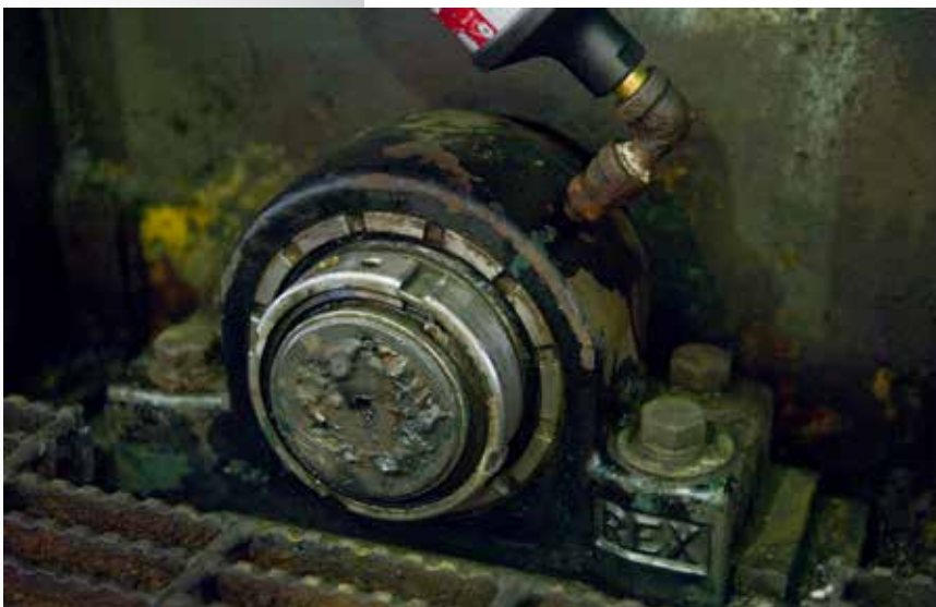
Rexnord ZA6215F adapter mount roller bearings with Shurlok technology incorporate a tapered locking sleeve to maintain bearing position on this quench tank.
