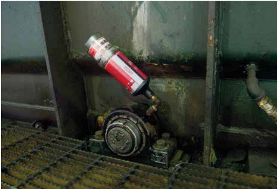
(Above) Bearings operate in a difficult environment on this quench tank application. Impact of tubes entering tank caused the roller shaft to move sideways with previous bearings.
