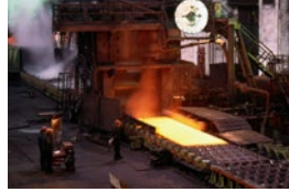
Steel mill roll out tables
