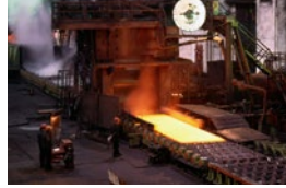
Steel mill roll out tables
