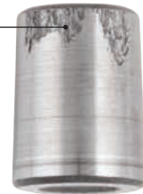
Geometric stress concentration damage
