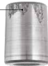
Geometric stress concentration damage
