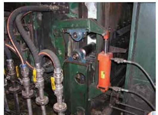
**Bearings on wringer side of the alkaline bath in the customer's galvanizing line operate in an extremely caustic environment. Previous bearings shown here had set screw mountings that loosened and damaged shafts, as well as seals that allowed the caustic solution into the bearings, which decreased bearing and lubricant life.**
