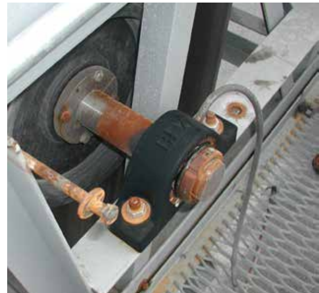
Rex 6000 Series SHURLOK Adapter Mounted Roller Bearing is easier to install on the bend roll of this conveyor and also handles misalignment better than the previous bearing.
