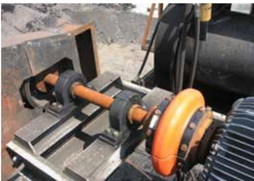
Closeup shows two Rexnord Bearings supporting jackshaft and Omega Coupling connecting motor to shaft.
