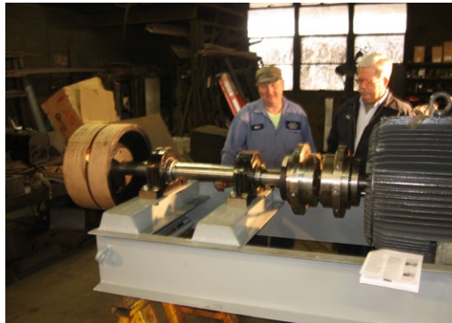
Jackshaft subassembly was put together in Eureka's shop before installation.
