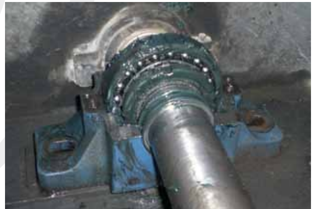
Previous split-block roller bearing design required field assembly that made it difficult to set clearances accurately and allowed contaminants to enter the bearing.
