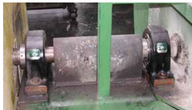
Shaft between V-belt drive and fan is supported by two bearings.
