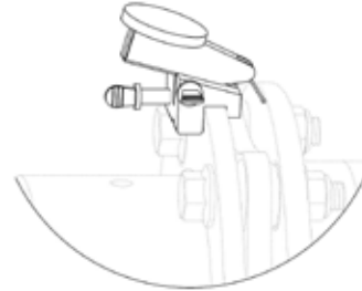
Figure 7 - Check angular alignment with Rexnord dial indicator method.
