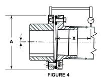
D. Angular Alignment — As the SN coupling is usually quite long, it is suggested to use the "Across the disc pack" procedure to correct the angular misalignment at each end. See Figure 2, 3, and 4.
