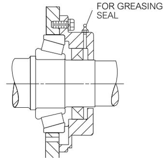
**CAUTION:** Rapid regreasing with a power grease gun can force grease inward past the seals and plug the oil drain back system causing seal leaks.
