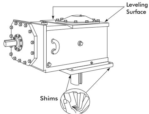
Check high speed shaft coupling alignment. If the coupling is misaligned, the bedplate is shimmed incorrectly. Re-shim bedplate and recheck high speed coupling alignment. If necessary, realign motor.
