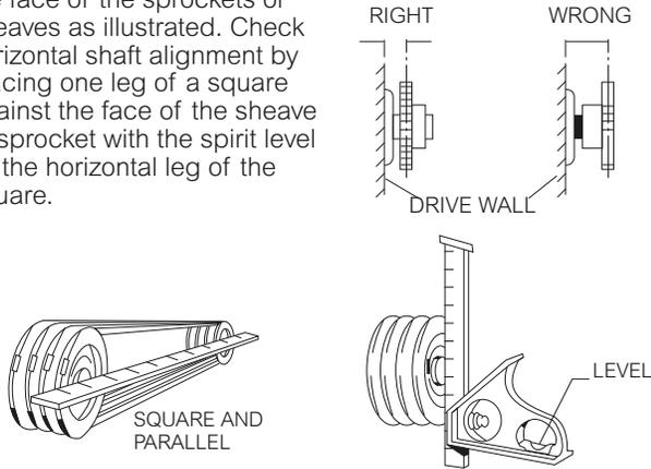
DO NOT over tighten belts or chains. Adjust chains to manufacturers' specifications. Adjust belts as follows: The ideal tension is the lowest tension at which the belt will not slip under peak load conditions. Check the belt tension frequently during the first 24 to 48 hours of run-in operation. Over tightening belts shortens belt and bearing life. Keep belts free from foreign material which may cause slippage. Inspect the V-belt periodically; tighten the belts if they are slipping.
