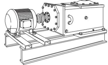
**GEAR DRIVE ALIGNMENT** — TAlign drive with driven equipment by placing broad, flat shims under all mounting pads. Start at the low speed shaft end and level across the length and then the width of the drive. Check with a feeler gauge to make certain that all pads are supported to prevent distortion of housing when drive is bolted down. After drive is aligned with driven equipment and bolted down, align prime mover to drive input shaft. Refer to Page 3 for coupling alignment.
