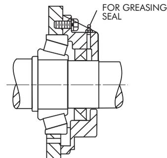
Periodically (at least every six months) depending upon the frequency and degree of contamination, purge contaminated grease from seals by slowly pumping fresh bearing grease thru the seal, **WITH A HAND GREASE GUN**, until fresh grease flows out along the shaft. Wipe off purged grease.
