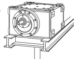
**GEAR DRIVE ALIGNMENT** — Align drive with driven equipment by placing broad, flat shims under all mounting pads. Start at the low speed shaft end and level across the length and then the width of the drive. Check with a feeler gauge to make certain that all pads are supported to prevent distortion of housing when drive is bolted down. After drive is aligned with driven equipment and bolted down, align prime mover to drive input shaft.
