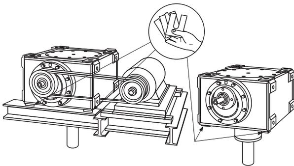
**LEVEL & ALIGN MOTOR PLATE** — Shim under the motor plate foot pads until level and all motor plate feet are in the same plane. Align low speed shaft with driven equipment. Bolt motor plate in place.
