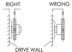
DO NOT over tighten belts or chains. Adjust chains to manufacturers’ specifications. Adjust belts as follows:
