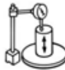
Check Axial Float Of Backstop Shaft With Dial Indicator
