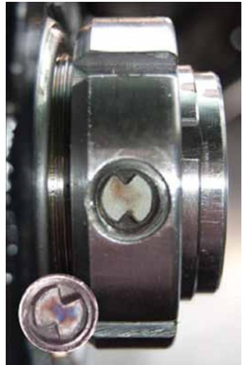
**(Right) Optical Strain Sensing (OSS) technology in new bearings changes color to tell the installer when the bearings have been correctly tightened to the shaft.**
