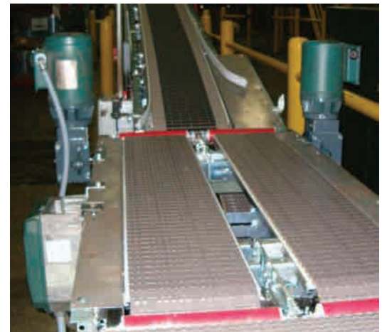
Ultramite UB Gear Units driving a multi-lane MatTop® conveyor
