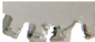
Continued use with broken grid elements will lead to complete destruction of hub teeth.
