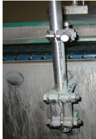
Evidence of hard water can often be seen by the limescale deposits on the sides of the conveyors and components.
