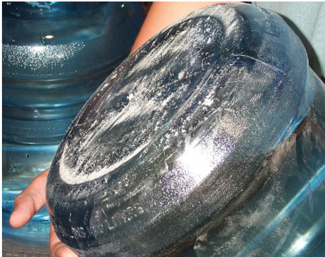
Product damage such as scuffing can occur without proper review.
