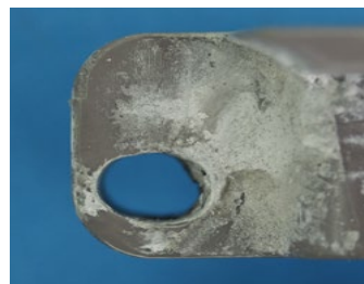
Increased component wear such as joint wear or elongation can be a result of water scale.
